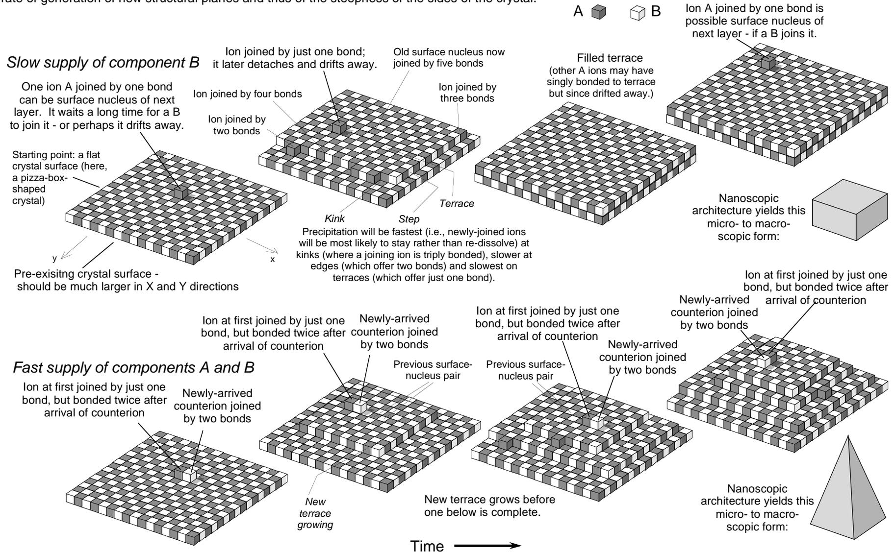
This model, in its general principles, explains why rapid precipitation promotes elongate crystals. Common examples are chalcedony (elongate) rather than quartz (equant) or elongate to fibrous calcite rather than equant calcite.
