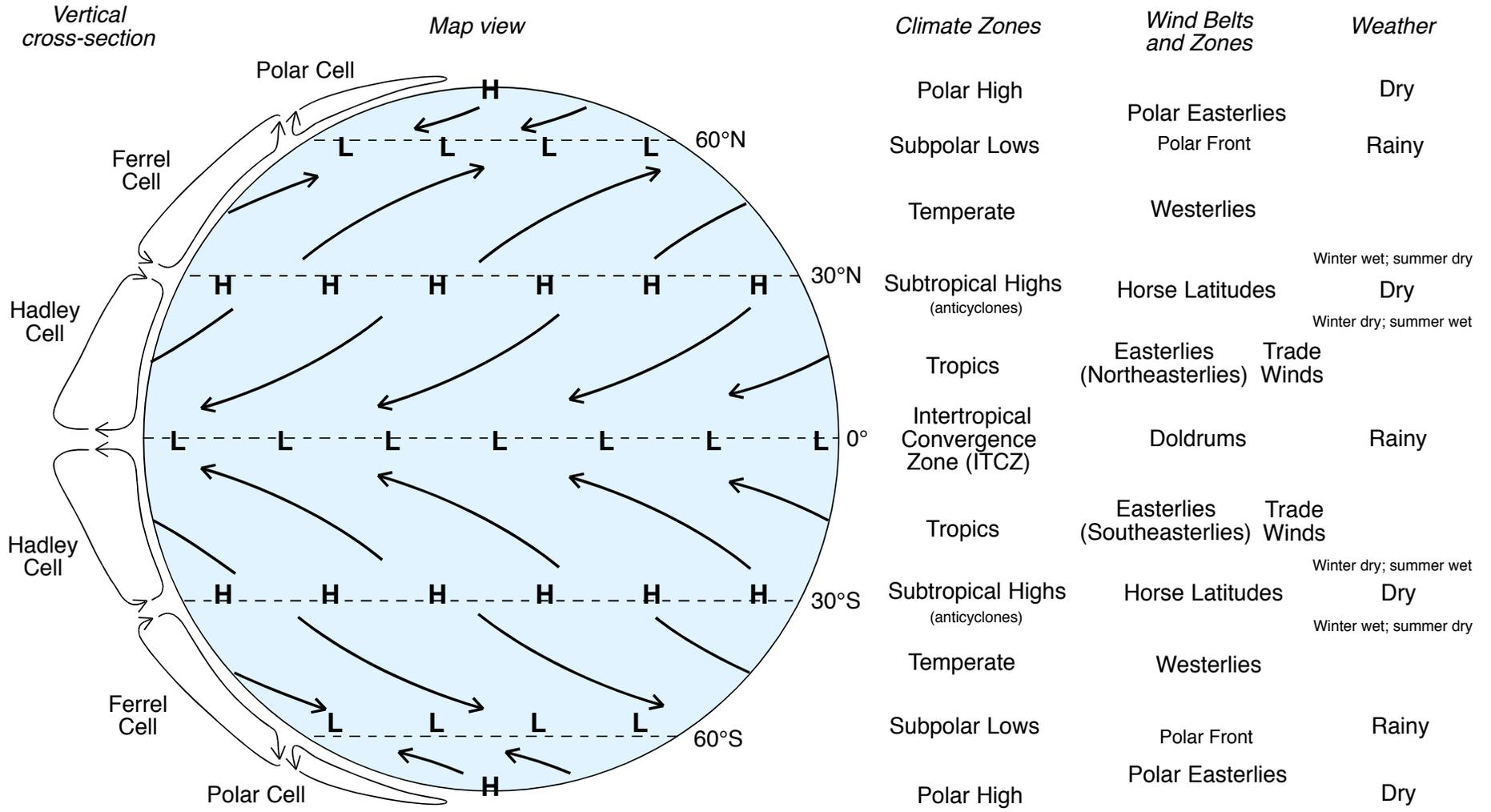
The diagram above is a typical schematic representation of Earth's surface atmospheric pressure, surface winds, and tropospheric circulation. It mimics diagrams in many introductory climatology and oceanography textbooks. Parts II to V of this series expand on this theme in a little more detail.
