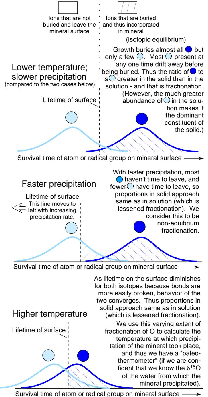
For each of the two isotopes, the curve above is the distribution of the probability (on the vertical axis) of survival for different lengths of time (on the horizontal axis).
